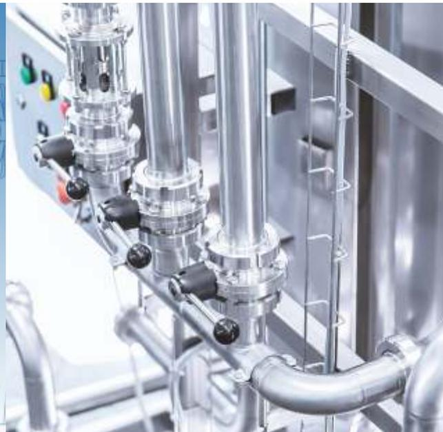
**ENG** Our machines meet the most demanding hygiene standards and support CIP machine cleaning process that is carried out in multiple stages (cleaning with an acidic agent, cleaning with an alkaline agent, disinfection and finally rinsing).
